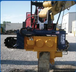
The new EM Series of vibratory pile driver/extractor represents the latest in high frequency technology. HMC has lead the industry in high frequency vibratory pile hammer technology and now has brought the same technology to the excavator mount vibratory pile driver/extractor market.
